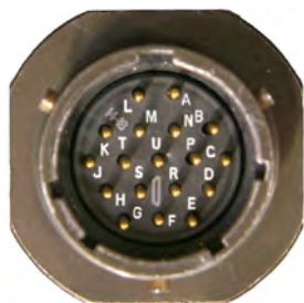
Figure 4. Pin Location Diagram. MS type Pigtail Cable Connector View from the front (mating) side
