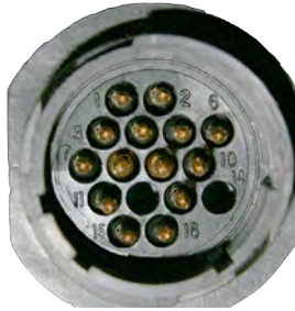
Figure 8. Pin Location Diagram. AMP type Pigtail Cable Connector View from the front (mating) side
