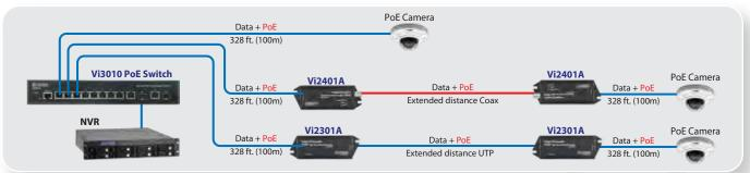
The Vi3010 is a high power PoE switch that provides eight 10/100/1G Ethernet ports plus 2 1G combo uplink ports. It is ideal for small to medium IP CCTV or IT network applications.
