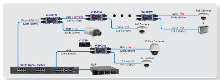
The Vi3003W is both a repeater and L2 3-port network switch providing drop and insert capability. It can be powered locally or from a power source and provide up to 60W to one camera at network speeds of 1000 Mbps.
