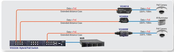
The Vi32226 is a 24-port managed PoE switch that can transmit Ethernet and PoE over Coax. They provide up to 36W PoE on each port. It is a cost effective and efficient solution for converting analog CCTV systems to IP systems.
