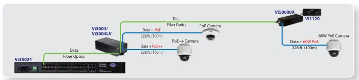
The Vi3004/Vi3004LV can provide can up to 60W PoE to high power cameras while transmitting data at long distances over fiber optics.
