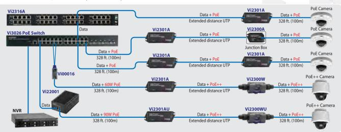
The Vi2300 series can transmit IP data and provide up to 72W PoE over extended UTP at distances up to 3,000 feet (914m) providing a cost effective method of powering, monitoring, and controlling your IP cameras
