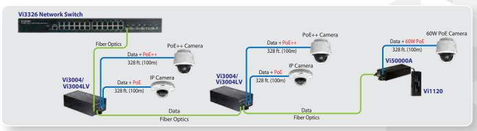
The Vi3004/Vi3004LV can provide up to 60W PoE on one port and 30W PoE on the second port. Their L2 network switching provide multiple drops over single cable runs and simplify installations. The Vi3004LV can use 24VDC or 24VAC power supplies.
