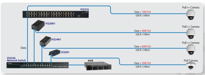
Vigitron's wide range of managed and unmanaged PoE Midspans can support virtually any size IP CCTV project requiring IEEE 802.3af to IEEE 802.3bt up to 90W PoE power.
