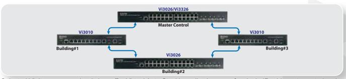
Selected Vigitron managed switches offer Virtual Auto Stacking, allowing use of a single IP address to control and monitor several switches on the same network without location restriction. It also eliminates the need for special stacking cables.
