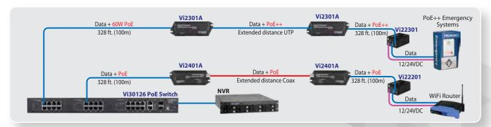
The Vi22201 and Vi22301 can be used along with Vigitron's Vi2300 or Vi2400 extender series to provide 12VDC or 24VDC at the remote locations to power non-PoE IP cameras or other IP devices requiring DC power input.
