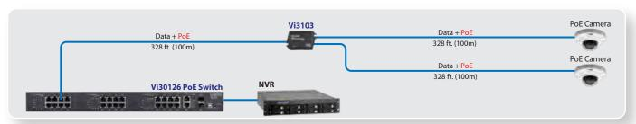
The Vi3103 is a 3-port PoE powered PoE switch that can be used to add an extra camera without new wiring or used as a drop and insert. It can be powered by PoE or a local power supply and provide up to 36W per port.
