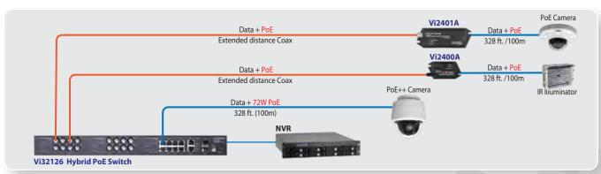
The Vi32026/Vi32126 can transmit Ethernet and PoE over Coax and UTP cables. They are cost effective and efficient in providing Ethernet and PoE for virtually any project with mixed types of cables. Ports 17-20 can provide up to 72W PoE power.
