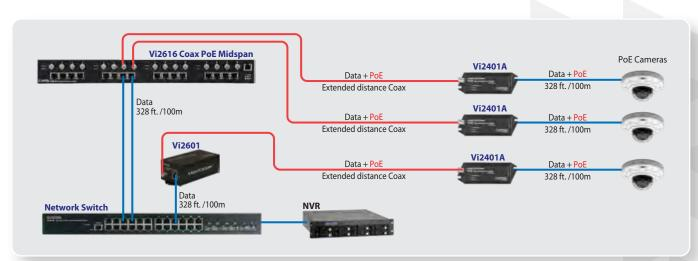
The Vi2608/Vi2616 provide PoE on up to 16 coax ports to power Vi2401A/Vi2400As and connected PoE cameras eliminating the need for local power sources. It is a perfect solution for parking lots, loading docks and perimeter applications. The Vi2601 provides Ethernet and PoE over long distances of coax and is ideal for smaller installations.
