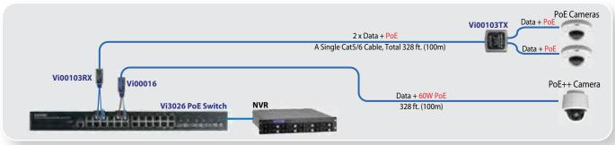
The Vi00016 can combine 2 PoE ports of any IEEE 802.3.at and provide up to 74W PoE power. The Vi00103 can transmit 2 IP streams and PoE over a single Cat5e/6.
