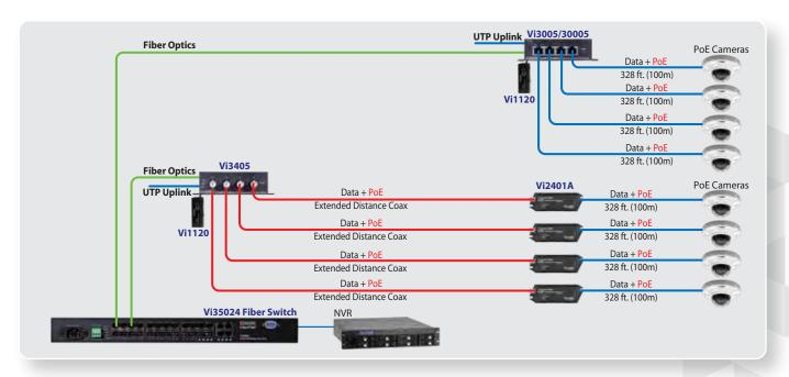
Vigitron's Vi3005 provides 4 10/100Mbps ports with PoE to connected devices. The Vi30005 provides 1000Mbps (1G) making it the perfect solution for connecting multiple network switches to minimize headend cable runs. Both Switches can be powered locally or by PoE eliminating the need for local power supply.
