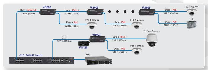
The Vi3003 is both a repeater and an L2 3-port network switch providing drop and insert capability. It can be powered by PoE or local power supply and providing up to 60W on one port and 36W on another port at 1000 Mbps. A local power supply can be used for powering 60W PTZ dome cameras.
