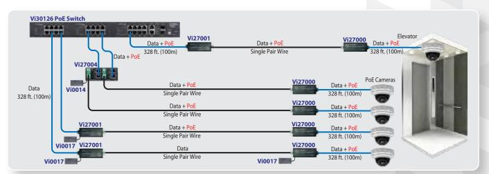
The Vi27000 series transmitter, receiver and IP cameras can be powered by a PoE switch.
