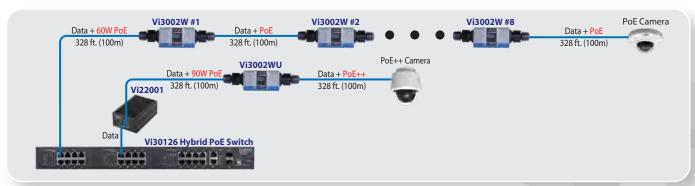
The Vi3002W/WU complies with IP67 standards eliminating the need for an extra outdoor housing. Their unique enclosure can easily be mounted to beams, buildings, or poles. Multiple Vi3002W/WUs, up to 8 units, can be used outdoor to extend Ethernet and PoE at desired distances.
