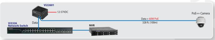
The Vi22601 is a compact and high power Midspan with 12VDC or 48-57VDC input that can provide PoE++ up to 60W for a wide variety of high power applications.
