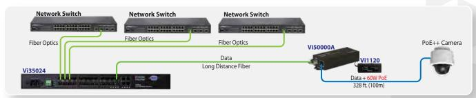
The Vi35024 can be used to combine data streams from several Network switches.
