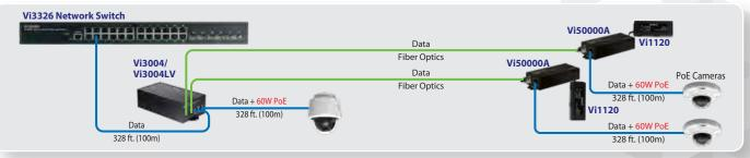
With Layer 2 network capacity, the Vi3004/Vi3004LV can be used to connect multiple cameras over Cat 5e/Cat 6 or fiber optics cables.
