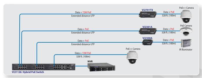
The Vi31026/Vi31126 can transmit Ethernet and PoE over standard and extended UTP cables. They are cost effective and efficient in providing Ethernet and PoE for virtually any project with new or existing extended UTP cables. Ports 1-4 and 17-20 can provide up to 72W PoE power.
