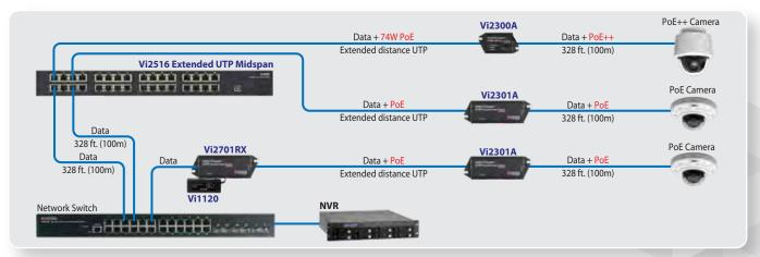
The Vi2516 provides PoE on up to 16 ports to power Vi2301A and connected PoE cameras eliminating the need for local power sources. It is an excellent solution for parking lots, loading docks and perimeter applications.
