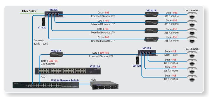
Vigitron's Vi3305 provides 4 extended UTP ports with a combination fiber and UTP uplink. The Vi3105 provides an extend UTP uplink with the ability to power both the switch and connected devices without the need for a local power supply. Each port is capable of providing up to 37W PoE depending on the input power supply.
