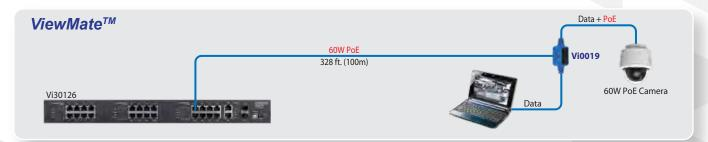
The Vi0019 is a wired PoE camera set up tool that provides PoE from a network to the camera while directing the video stream from the camera to a laptop. It enables the installer to see the image and set up the camera. It can pass through up to 60W PoE and also provides LED indicators that show the status of PoE. The Vi0019 uses PoE and does not require a separate power supply.
