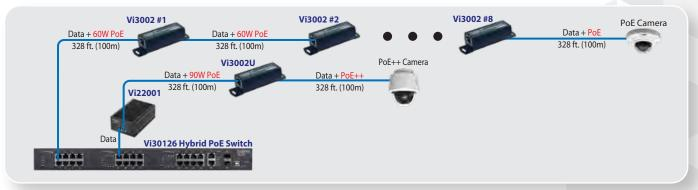
Multiple Vi3002/Vi3002Us, up to 8 units, can be cascaded to extend Ethernet and PoE at desired distances.
