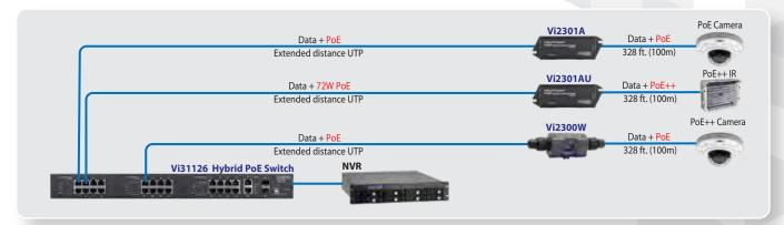
The Vi31126 is a 24-port managed Hybrid PoE switch than can transmit Ethernet and PoE over standard and extended distance UTP cables. It provides up to 36W PoE on each port and 72W PoE on ports 1-4 and 17-20. It is a cost effective and efficient solution for converting analog CCTV systems to IP or new installations.
