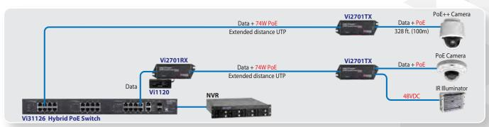
The Vi2701TX can provide IP video and PoE plus a 48VDC output to power auxiliary devices such as IR Illuminators.
