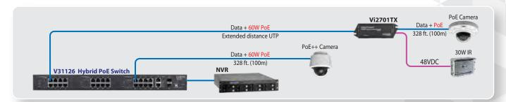
The Vi2701TX is capable of accepting 60W PoE input at long distances and eliminate the need for local power supplies. It can provide PoE output to the cameras as well as DC voltage to accessories.
