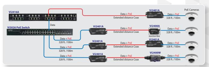
The Vi2400 series can transmit IP data with up to 37W PoE over existing coax at distances up to 1,800 feet (545m) providing a quick and cost effective method of converting analog CCTV to IP systems.
